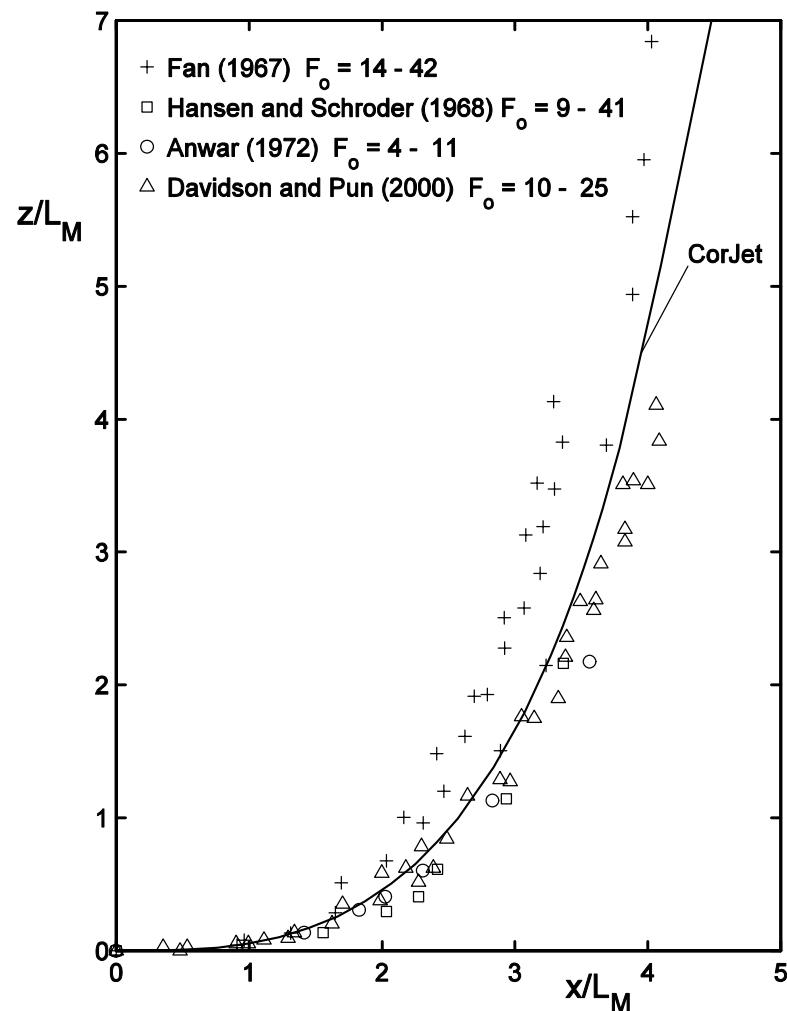
**Horizontal buoyant jet in stagnant ambient:** Normalized vertical trajectory as a function of  $L_M$
