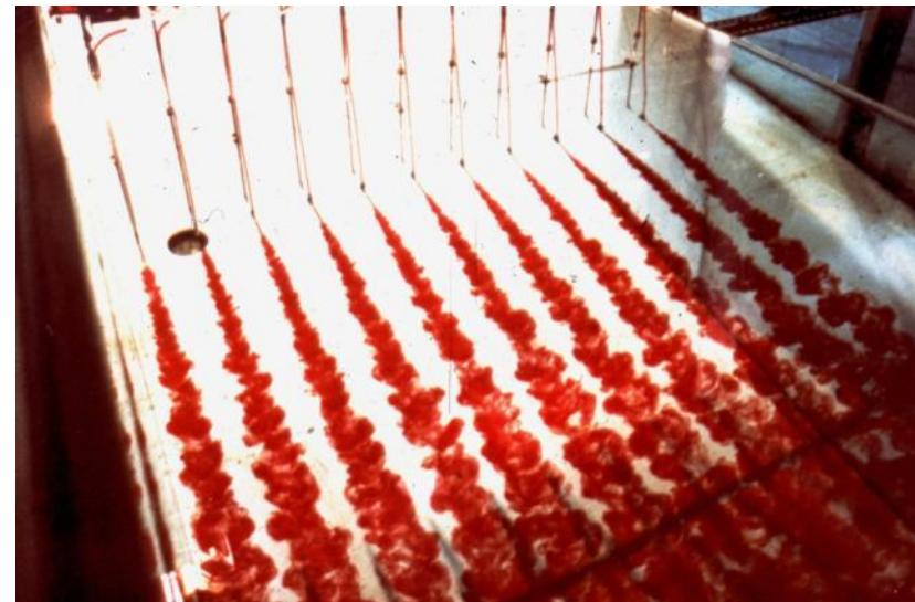
Regular merging processes for a unidirectional diffuser design. (a) Schematic side view and (b) top view under stagnant ambient conditions, (c) photograph of merging under co-flowing ambient conditions (courtesy of I.R. Wood)
