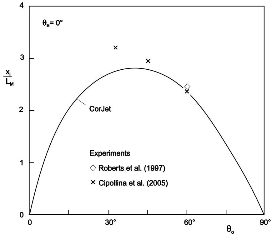
Jet properties at impingement point for zero offshore slope ( $\theta_B = 0^\circ$ ).
