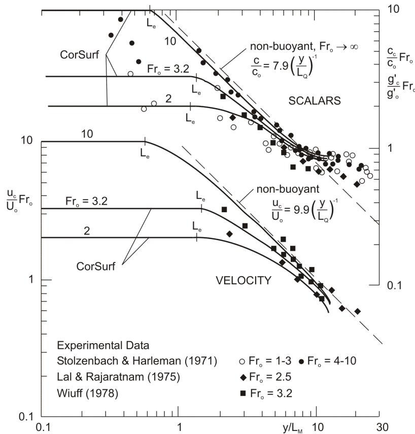
Surface buoyant jet in stagnant ambient. Comparison of laboratory experimental data with predictions of integral model CorSurf (with aspect ratio  $A = 0.5$ ). Normalized centerline velocity  $(u_c/U_o) Fr_o$  and centerline concentration  $(c_c/c_o) Fr_o$ , or centerline buoyancy  $(g'_c/g'_o) Fr_o$  as a function of offshore distance  $y/L_M$
