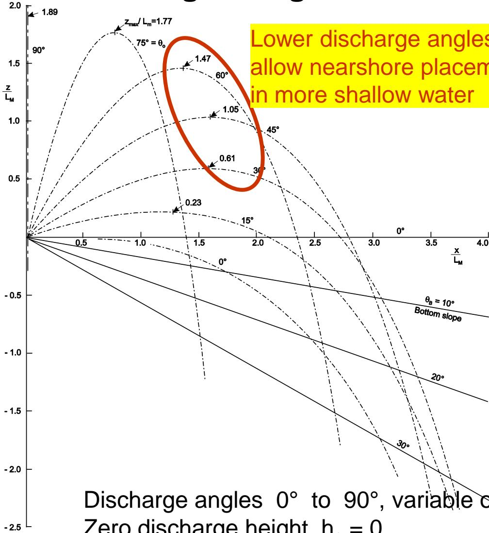
Discharge angles  $0^\circ$  to  $90^\circ$ , variable offshore slopes  $\theta_B$  from  $0^\circ$  to  $30^\circ$ .
