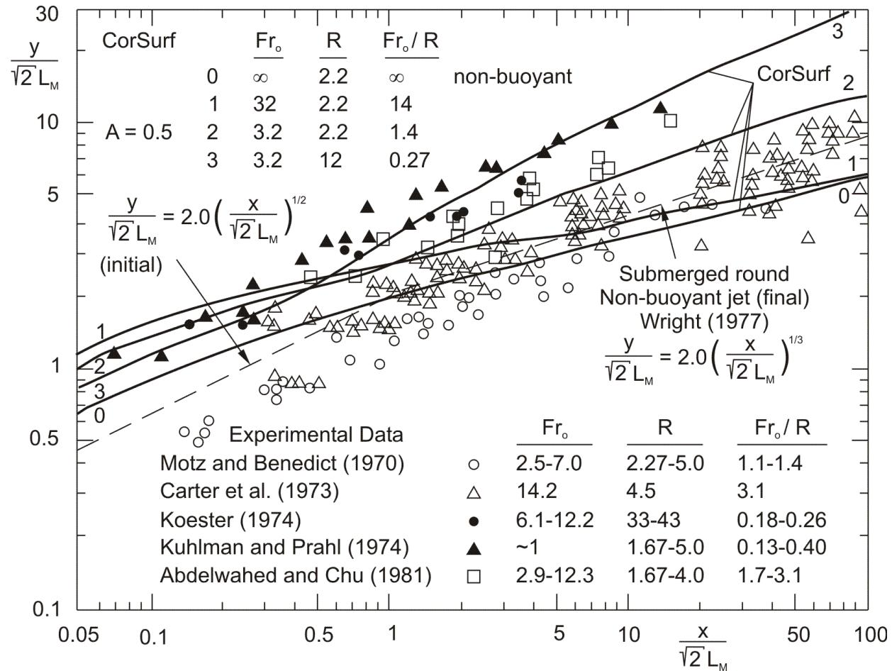
Free surface buoyant jets in ambient crossflow (flow class FJ1 and Fj2). Comparison of laboratory data with predictions of integral model CorSurf (with aspect ratio  $A = 0.5$ ). Normalized jet centerline trajectories  $y/(\sqrt{2}L_m)$  as a function of longshore distance  $x/(\sqrt{2}L_m)$ . Data and model predictions show dependence on ratio  $Fr_o/R = L_M/L_m$
