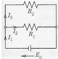
$$I_2 = E_0/R_1, \quad I_3 = E_0/R_2, \quad I_1 = (R_1 + R_2)E_0/(R_1R_2)$$
