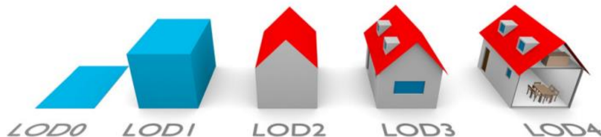
Fig. 1. The five LODs of CityGML 2.0. The geometric detail and the semantic complexity increase, ending with the LOD4 containing indoor features.
