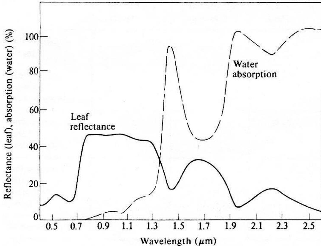
**Figure 5-9** The inverse relationship between leaf reflectance and water absorption. The water-absorption curve represents the amount of absorption caused by a layer of water 1 mm deep. (After Hoffer and Johannsen.<sup>3</sup>)
